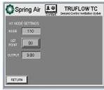
The **NODE** window displays the temperature received from the J-couple on the hood. The **SET POINT** icon
