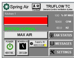
This picture shows the POWER is ON for single Kitchen (Green). Systems is running at 100% speed and CFM. (Bar is RED. 100% of MAX and 60.0 Hz)
