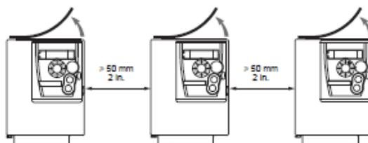
Free space  $> 50$  mm (2 in.) on each side. Vent cover should be removed for operation at surrounding air temperature above  $50^\circ\text{C}$  ( $122^\circ\text{F}$ ). The degree of protection becomes IP20
