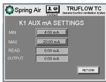
Touching the **K1 AUX mA** icon displays the setting screen. From here, you can adjust the **MIN** and **MAX** mA settings that are sent to the Auxiliary Output on terminals E and F in the RPD panel.
