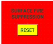
To resume normal operation, the fire suppression system and TC panel unit will need to be reset. The fire suppression contractor will need to reset the suppression release to open the micro switch that signals the tripped status. Once this has been reset, you will need to go to the MESSAGE screen. You will see the Surface Fire Suppression RESET button. Touching this button will reset and allow normal operation of the TC system.
