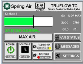
The HMI (Human Machine Interface) is the point of contact for operating the TruFlow TC system. The information displayed is the normal operating condition.
