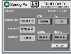
This screen displays the running frequency of the VFD, the actual voltage at the VFD and the running amps for Kitchen 1. The CFM is the design CFM and the HP is the motor size on Horse Power.
