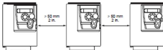
Free space  $> 50$  mm (2 in.) on each side, with vent cover fitted. Mounting type A is suitable for drive operation at surrounding air temperature less or equal to  $50^\circ\text{C}$  ( $122^\circ\text{F}$ ).
