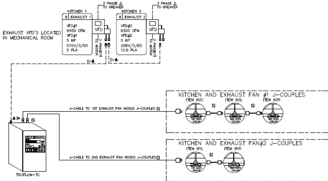
*Truflow-TC panel with two kitchens, 5 hood collars, two exhaust VFD and supply fan Control signal only*
