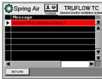
When the control panel senses an input for any reportable alarm or message, the **EXCLAMATION** screen
